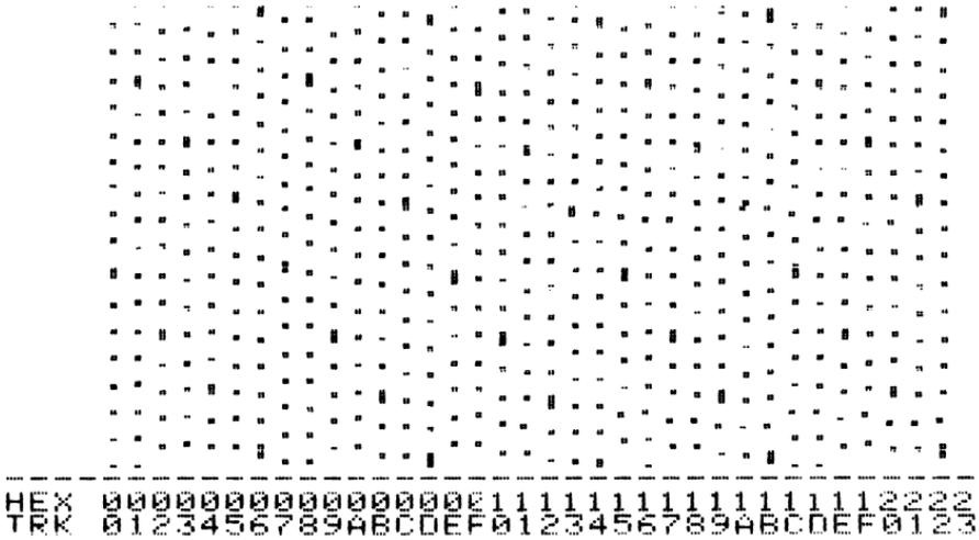
Each track is plotted in a vertical line over the track number. Any normal 16-sector disk will produce a display similar to this. The dots are the sync fields between the sectors. The short stripe on each track is the longer sync field at the start of the track.
