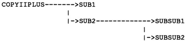
This diagram shows that the main, or “root”, directory (which goes by the volume name “COPYIIPLUS”) has two subdirectories, named SUB1 and SUB2. In addition, the subdirectory SUB2 contains two subdirectories of its own, called SUBSUB1 and SUBSUB2. (This is called a “tree” diagram because the subdirectories extend from the “root” directory like branches of a tree.)
